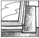
Along the side, the first layer of felt, which lies over the last course of shakes, is run under the L gasket. The first shake on the side is also positioned under the L gasket.
