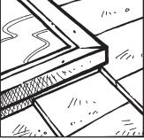
At the top, felt and shakes are placed over the L gasket. Continue to apply shakes up the roof.
