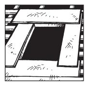
Lay down a base layer of felt paper around the opening.
