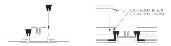
**Step 10** – Bend down glazing over rib & engage into outer glazing slot in header QR sill. Outer glazing should rest on top of rib divider gasket.
