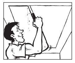
Cut the ceiling opening with a saw or sheetrock knife. Cut through any ceiling joists within the opening and support temporarily. Frame the opening with headers and trimmer joists as needed. NOTE: To maintain the structural integrity of the roof and ceiling, double headers, rafters and joists may be necessary.
