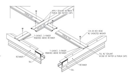
**STEP-15:** After unit has been completely fastened, proceed to seal all joints with sealant.
